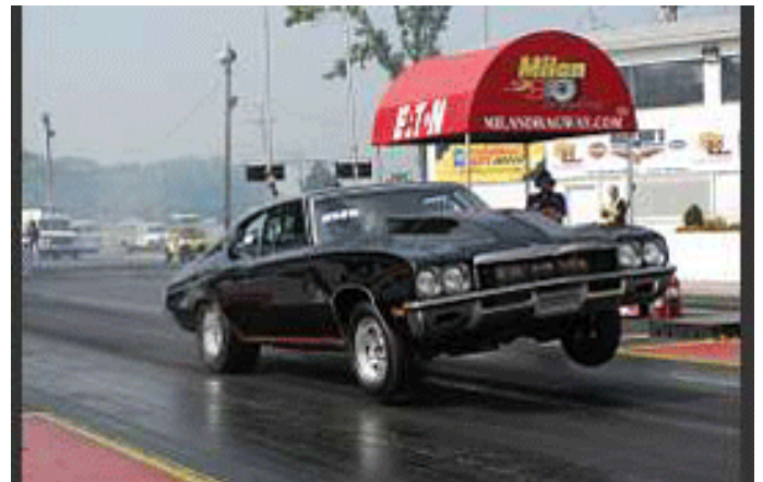
Bobb Makley 535 Procharged, flat tappet cammed, stage 2 headed, 8.80's @ 153 MPH at 3700LBS and stock suspension.
