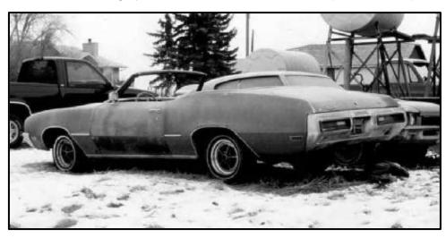
kept rust from starting in the passenger floor area (which is a really common problem on convertibles). Also, they had removed the floor drain plugs, which was a good idea. You can see the front fenders have the usual rot in the lower corners (I have already found some fenders) and the lower quarters have some rust as well...pretty minor stuff for a 28 year old convertible.
