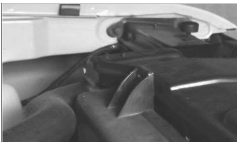
Pictures showing the upper mounting tabs of a 1970 big block (left) and 1971-72 big block (right) fan shroud. (Note the position of the leading edge of the fan shroud.)
