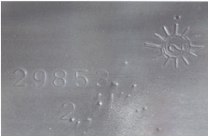
Here are pictures of the left & right upper mirror housing casting numbers and date code clocks.
