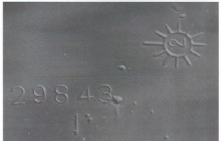
Here are pictures of the left & right upper mirror housing casting numbers and date code clocks.
