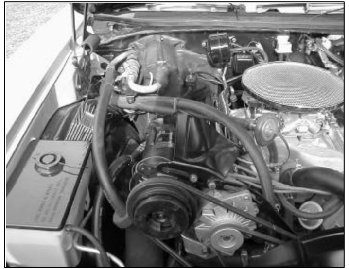
These pictures show some close-ups of the engine. You can see the Motion emblems on the valve covers, Mickey Thompson Headers, Edelbrock B4B intake, Holly 3-bbl carb, and the “Fly Eye” air cleaner. The picture on the right also shows the location of the Phase III ignition system. Normally this would have been mounted on the firewall, but the AC system made the firewall too “busy”, so the techs mounted it on the right inner fender.
