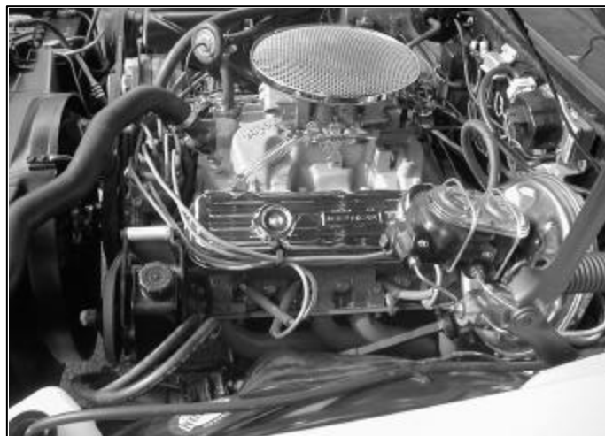
These pictures show some close-ups of the engine. You can see the Motion emblems on the valve covers, Mickey Thompson Headers, Edelbrock B4B intake, Holly 3-bbl carb, and the “Fly Eye” air cleaner. The picture on the right also shows the location of the Phase III ignition system. Normally this would have been mounted on the firewall, but the AC system made the firewall too “busy”, so the techs mounted it on the right inner fender.
