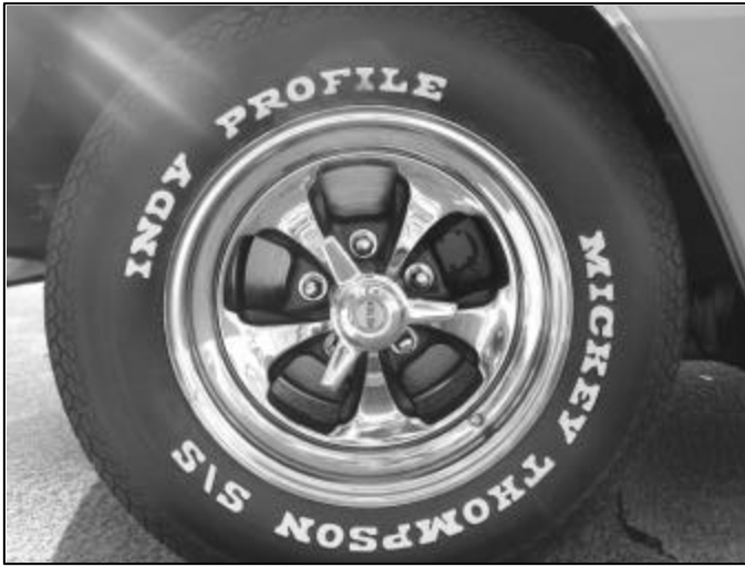
Close-up of the Keystone Mag wheels with the "Motion" Spinners, and Mickey Thompson tires
